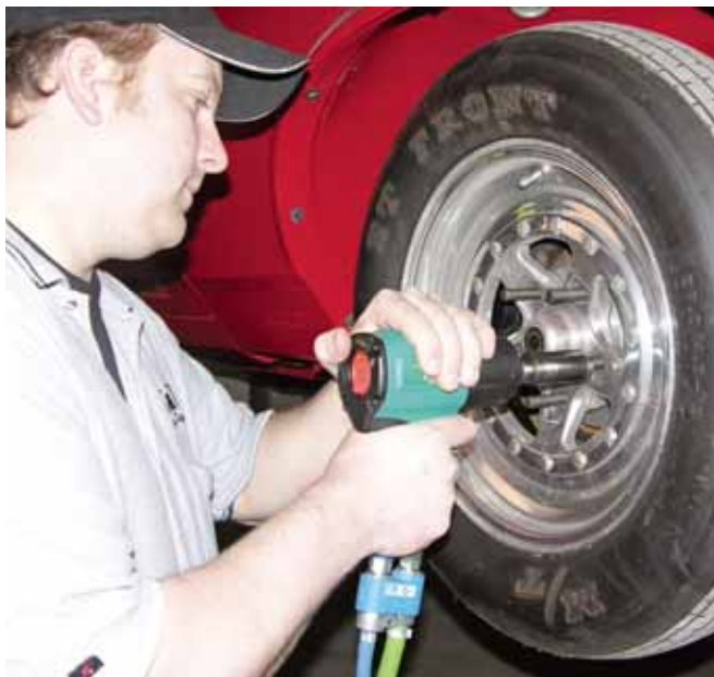
Instead of compressed air being released through the handle of an air gun, a second hose recirculates it to the intake side of the compressor.
