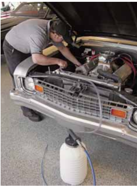
The DX12 evacuator can be used to remove coolant, transmission fluid, engine oil and gear oil.
