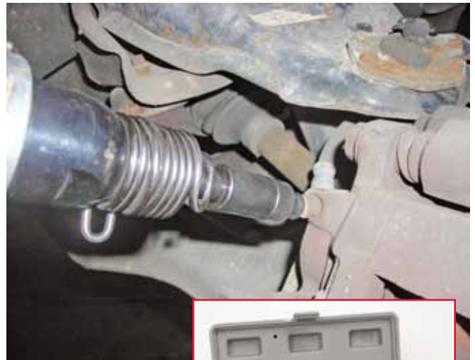
The Vacula Brake Caliper Rescue Tool is designed to remove frozen bleeder valves.
